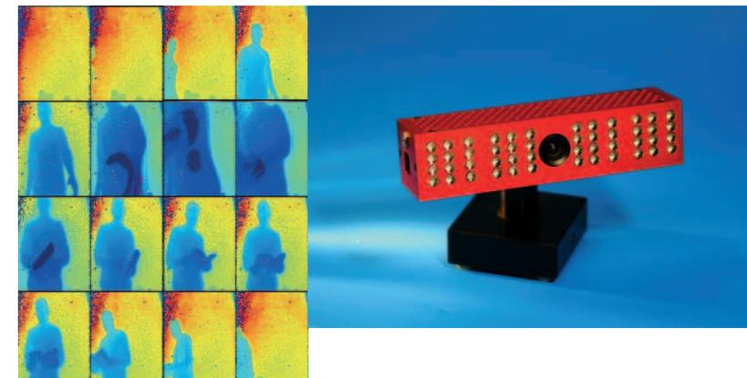
Fig. 3.5.6 Left: A few scenes out of a 3D movie acquired with an optical time-of-flight range camera. The distance images are color-encoded (dark blue = 10 cm; red = 750 cm); right: Miniaturized optical time-of-flight range camera with millimeter resolution, based on a custom CCD/CMOS image sensor with smart pixels © CSEM
