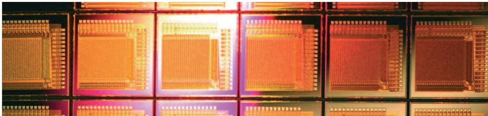
Fig. 3.5.9 Today's high-performance CIS (CMOS Image Sensor) technology is the basis for a large range of custom functionality image sensors © CSEM
