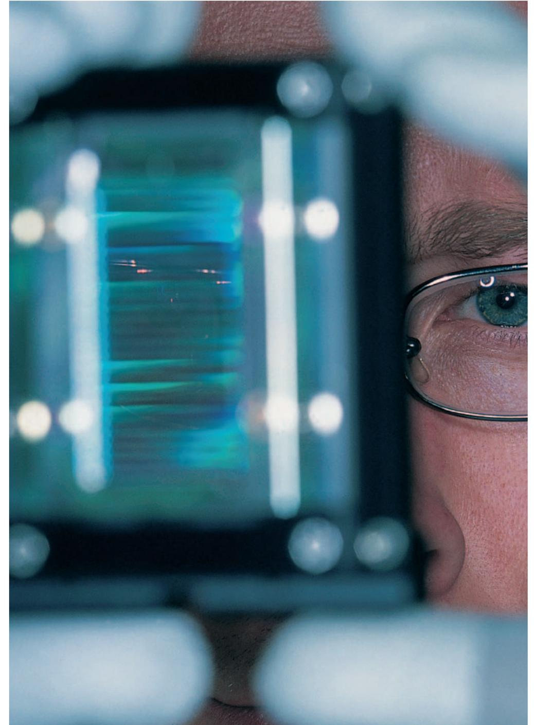
Fig. 3.6.7 Diode lasers are the most efficient artificial light sources existing. Due to their high efficiency and long service life, they have proved a success in many applications. The extremely compact diode lasers are increasingly gaining importance as light sources for direct treatment in industry and medicine and as highly efficient pumping sources in solid state lasers © Jenoptik
